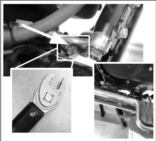
**3** Remove the front engine mount bolt (arrowed), Washer (3) and U nut (1). Assemble the front mount bracket (2) as shown, leaving the bolt loose at this stage.
